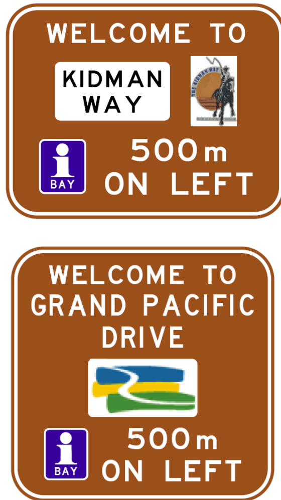
Figure 3.59 Examples of TOURING ROUTE WELCOME (G11-215) signs
