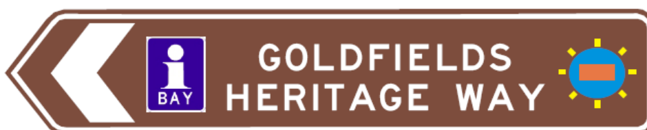
Figure 3.53 Example of TOURING ROUTE INFORMATION BAY ENTRY (G11-215) sign
