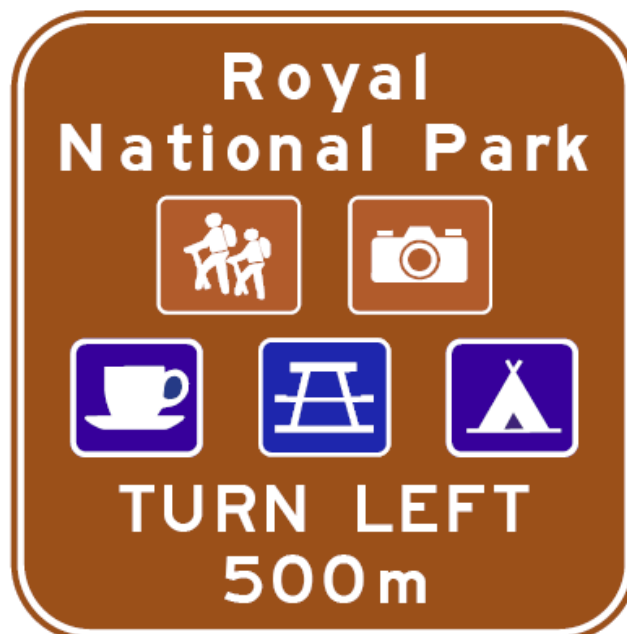
Figure 3.18 Example of an ADVANCE DIRECTION (G11-209) sign
