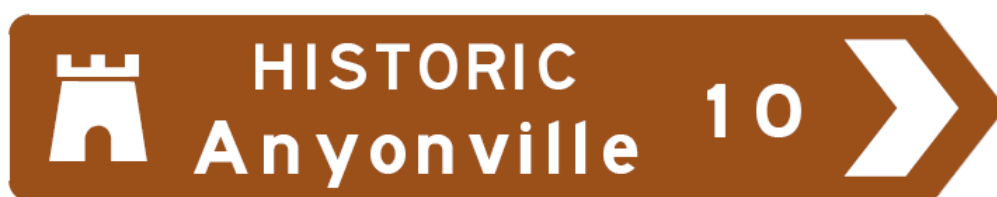
Figure 3.16 Example of FINGERBOARD (G3-201) for an historic town or village
