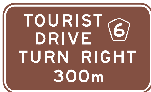
Figure 3.37 Example of ADVANCE (G8-207) sign
